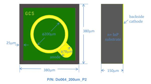
Attention: InP brittle material and electrostatic sensitive device, observe precaution for handling.
