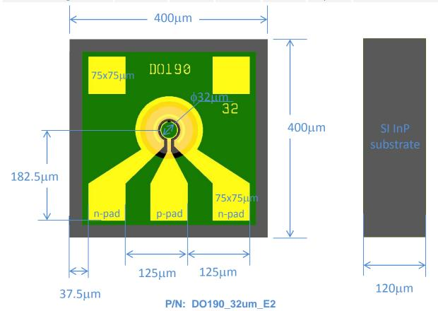
Attention: InP brittle material and electrostatic sensitive device, observe precaution for handling.
