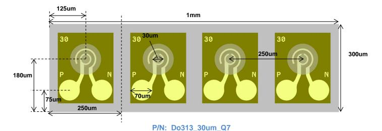
Attention: GaAs material and electrostatic sensitive device, observe precaution for handling.
