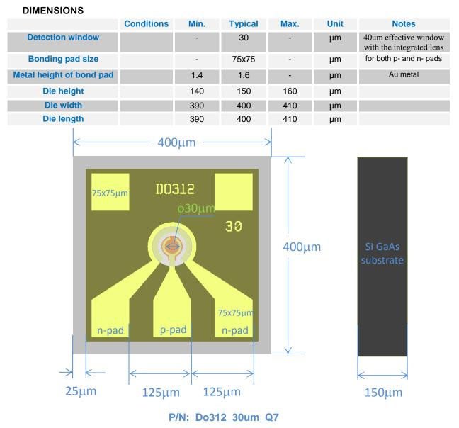
Attention: GaAs material and electrostatic sensitive device, observe precaution for handling.
